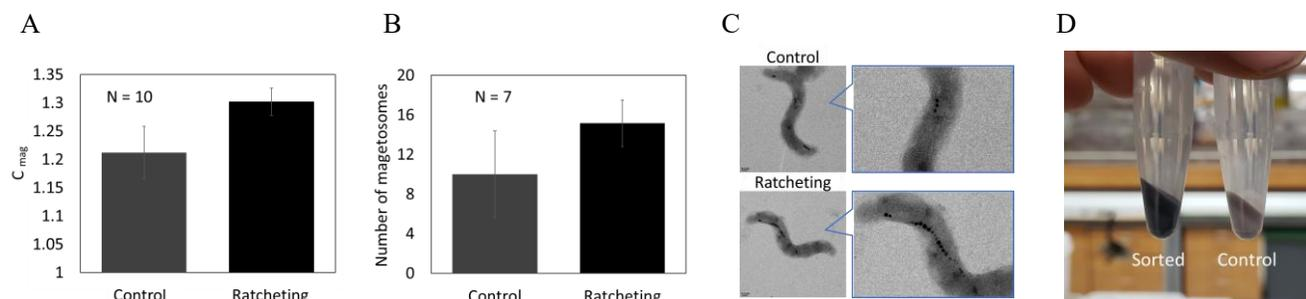
Figure 4: A-B)  $C_{\text{mag}}$ , a measure of magnetic content and number of magnetosomes is increased after sorting C) TEM Picture of AMB-1 control and after sorting D) Total production of magnetosome from control and sorted population
