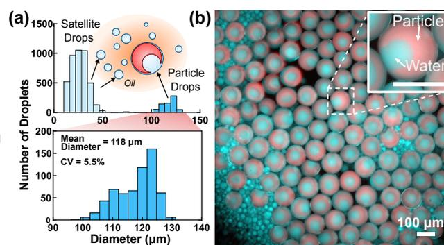
**Figure 3.** (a) Droplet size analysis after emulsification shows two distinct subpopulations: smaller heterogeneous satellite drops and monodisperse particle-drops. (b) Fluorescent image of particle-drops with dye added to water phase to aid in visualization.
