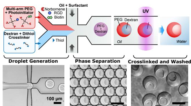
**Figure 2.** Fabrication of cavity-containing particles using an aqueous two-phase based approach. UV reactive PEG and photoinitiator is coflowed with dextran in a flow focusing device. PEG and dextran undergo phase separation and are crosslinked via UV light downstream. Particles are collected and washed for later use.
